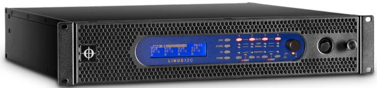
The LINUS12C is a four channel networkable DSP amplifier delivering 4x 3000 W of virtually distortion-free power in a light weight 19"/2U package. The 4 audio inputs are selectable from analog, AES3 or LiNET digital audio and are routable to any of the 4 outputs.
