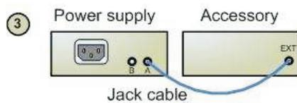
Or connect two accessories using two jack cables as shown in diagram 2.
