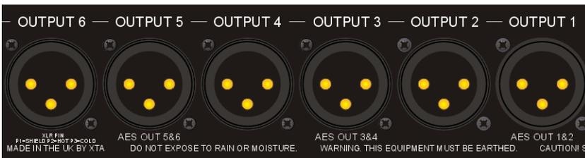
**Audio Outputs:** 3 pin XLR sockets are provided for each channel. All are fully balanced, pin 2 hot, 3 cold, 1 screen.
