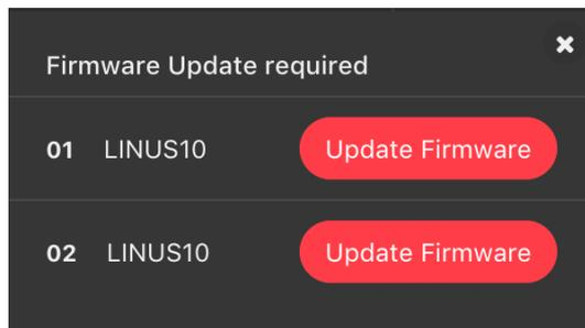
*Note – If after pressing the 'Update Firmware' button, it reappears after a short period of time, power cycle the amplifier. Once the 'Update Firmware' button is pressed, the amplifiers will disappear out of the discovery list. Please wait at least 30 seconds for the amplifiers to show up in the discovery list.*
