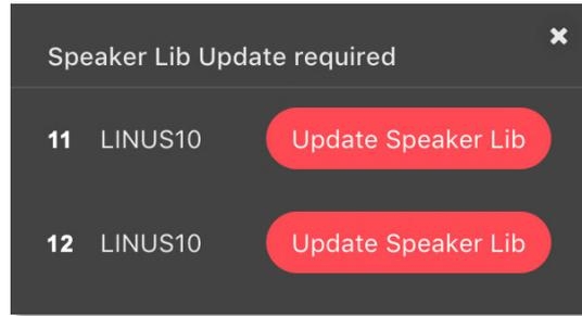
*Note – If the amplifier that was the ‘Slave’ does now show up now in the discovery list with the “Update Speaker Lib” button, you forgot to perform the step marked ‘Important’ above; whereby you should set all devices to Master & not adjust the ID. To recover the amplifiers, it is now necessary to place the master and slave in Hardware Update mode, then push the firmware to both of the amplifiers one at a time, prior to restarting this above procedure.*
