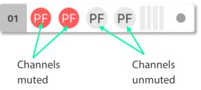
When the channel mutes are off, output meters are displayed in green behind the suffix. The output meters are calibrated in dB relative to the loudspeaker's full RMS output potential on a per-channel basis.
