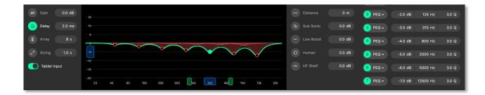
All group tuning parameters are enabled and disabled by clicking on the corresponding icon. A greyed-out icon means the parameter is disabled. A green icon means the parameter is enabled.
