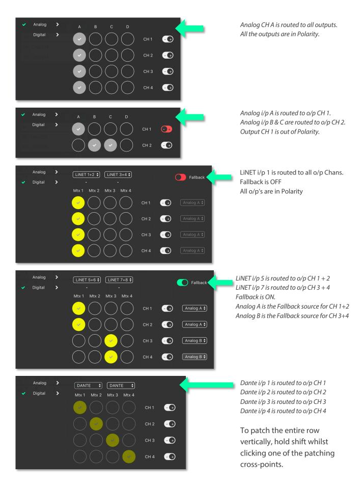
Note – The Dante patch is fixed one to one in the Firmware. To adjust the routing of the Dante, please use Audinate's Dante Controller.
